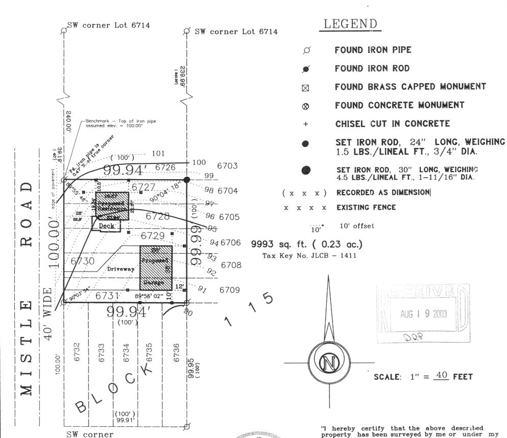
property has been surveyed by me or under my direction and that the above map is a true representation thereof and shows the size and location of the property, its exterior boundaries, the location of all visible structures and dimensions of all principal buildings thereon, boundary fences, apparent easements, roadways and visible encroachments, if any."
